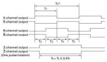
$<sup>*</sup>T_0$  is the average time for one encoder rotation when the encoder is rotated at a constant speed.
