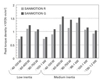
Fig. 3 Comparison of peak torque density
