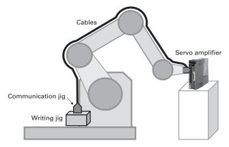
Fig. 14 Automatic writing using robot
