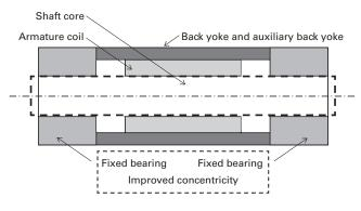
Fig. 6 Cross section view of new product's stator
