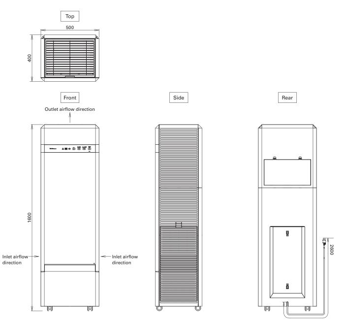
Fig. 4 Dimensions of San Ace Clean Air 9AP type (Unit: mm)
