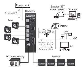
Fig. 4 San Ace Controller system configuration example
