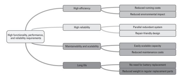
Fig. 2 Functionality, performance, and reliability required of UPS
