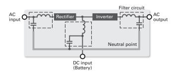
Fig. 3 Simplified A23D circuit block diagram
