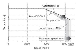
Fig. 4 Comparison of servo motor torque-speed characteristics
