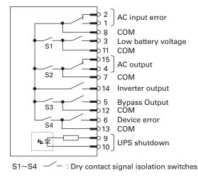
Fig. 7 Dry contact output interface
