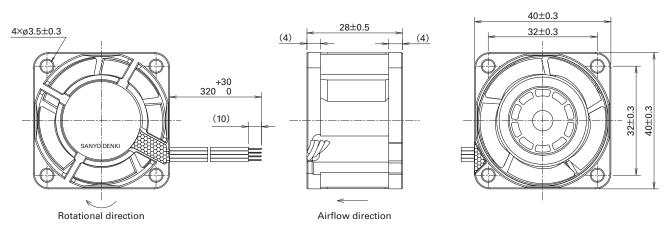
Fig. 5 Dimensions of 40 × 40 × 28 mm San Ace 40W 9WPA type (Unit: mm)
