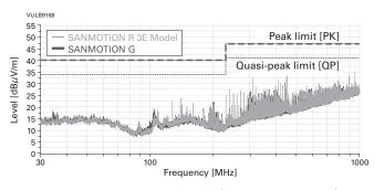
Fig. 7 Radiated emissions (10 m, horizontal)
