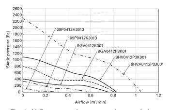
Fig. 1 Airflow vs. static pressure characteristics of our 40  $\times$  40  $\times$  28 fans
