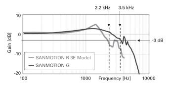
Fig. 5 Comparison of frequency response in speed control system
