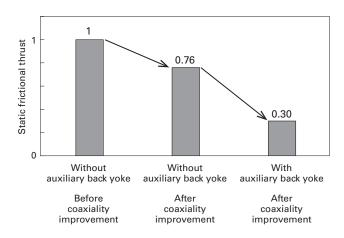
Fig. 8 Comparison of static frictional thrust
