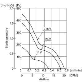
Fig. 13 Airflow vs. static pressure characteristics of  $40 \times 40 \times 28$  mm San Ace 40W 9WPA type 24 V, low-speed model
