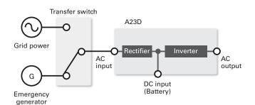
Fig. 5 Emergency power supply system
