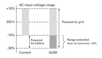
Fig. 4 Wide input voltage range
