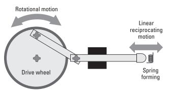
Fig. 3 Simple linkage configuration
