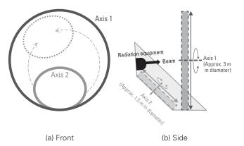
Fig. 5 Beam irradiation direction servo mechanism and size
