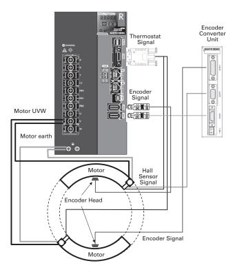
Fig. 6 Image of encoder signal redundancy
