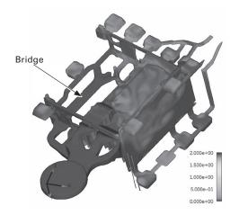
Fig. 16 Die casting fluid analysis (with bridge)
