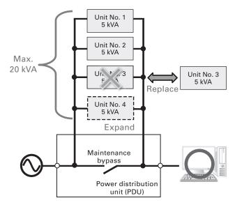
Replacement or expansion can be performed without interrupting power supply to the load.
