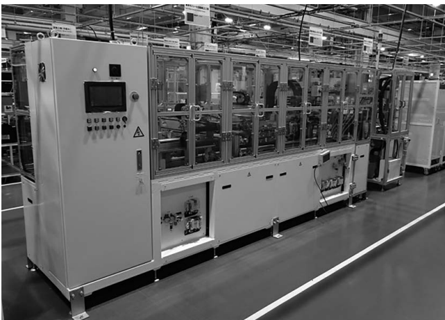
Fig. 7 The SANUPS LiB Pack automated assembly/ inspection equipment
