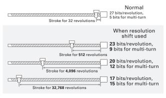
Fig. 8 Encoder resolution shifting illustrations
