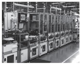
Fig. 10 Automated production line for DC servo motors
