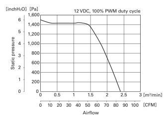
Fig. 3 Airflow vs. static pressure characteristics of the 60  $\times$  60  $\times$  76 mm *San Ace 60L* 9CRLB type
