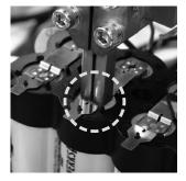
Fig. 8 Resistance welding
