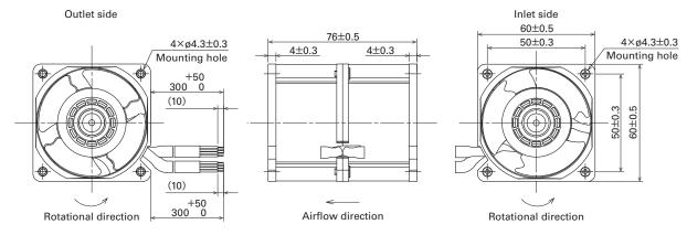
Fig. 2 Dimensions of 60 × 60 × 76 mm San Ace 60L 9CRLB type (Unit: mm)
