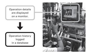
Fig. 7 Production guidance system
