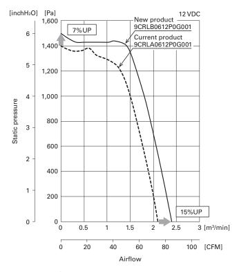
Fig. 7 Airflow vs. static pressure characteristics of the new and current products
