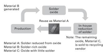
Fig. 10 Solder recycling workflow
