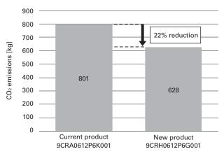
Fig. 8 CO<sub>2</sub> emissions comparison using our LCA calculation software (40,000 hours, when operating with the same operating airflow)
