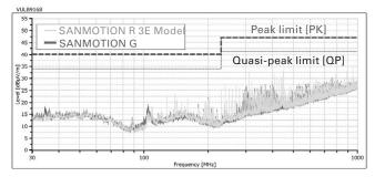
Fig. 2 Radiated emissions (10-m method, horizontal axis)
