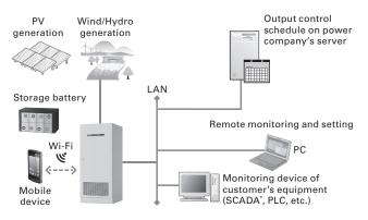
\* SCADA (Supervisory Control and Data Acquisition): industrial equipment control and monitoring systems
