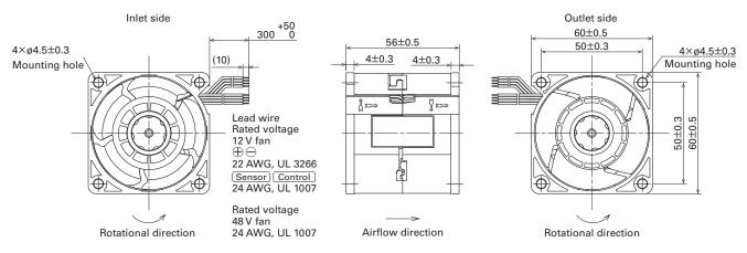
Fig. 2 Dimensions of  $60 \times 60 \times 56$  mm San Ace 60 9CRH type (Unit: mm)
