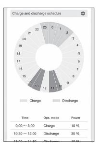
Fig. 12 Charge/Discharge schedule setting screen
