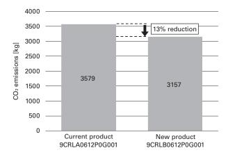
Fig. 9 CO<sub>2</sub> emissions comparison using our LCA calculation software (100,000 hours, when operating with the same operating airflow)
