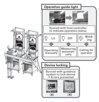
Fig. 8 Overview of operator guidance system
