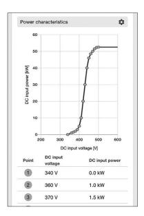
Fig. 11 Generator power curve setting screen
