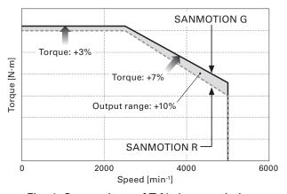
Fig. 4 Comparison of T-N characteristics of medium-inertia motors
