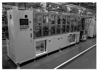
Fig. 7 The SANUPS LiB Pack automated assembly/ inspection equipment
