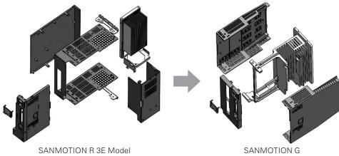
(Front resin cover, sheet metal, and extruded fins)
