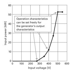
Fig. 3 Generator power curve settings illustrated
