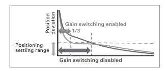
Fig. 6 Positioning settling characteristics
