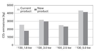
Fig. 12 Comparison of servo motor CO<sub>2</sub> emissions
