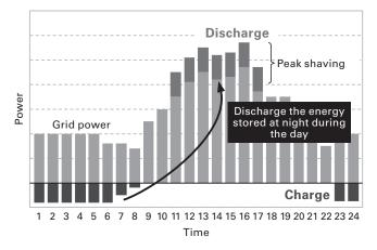
Fig. 4 Schedule-based charge/discharge control illustrated
