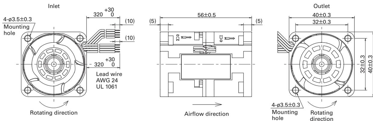
Fig. 2: Dimensions of the new model (unit: mm)
