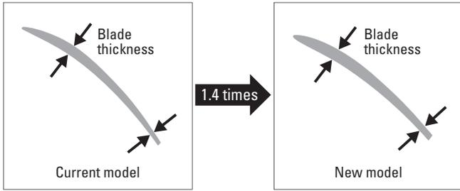
Fig. 5: Comparison of current and new model blade thicknesses
