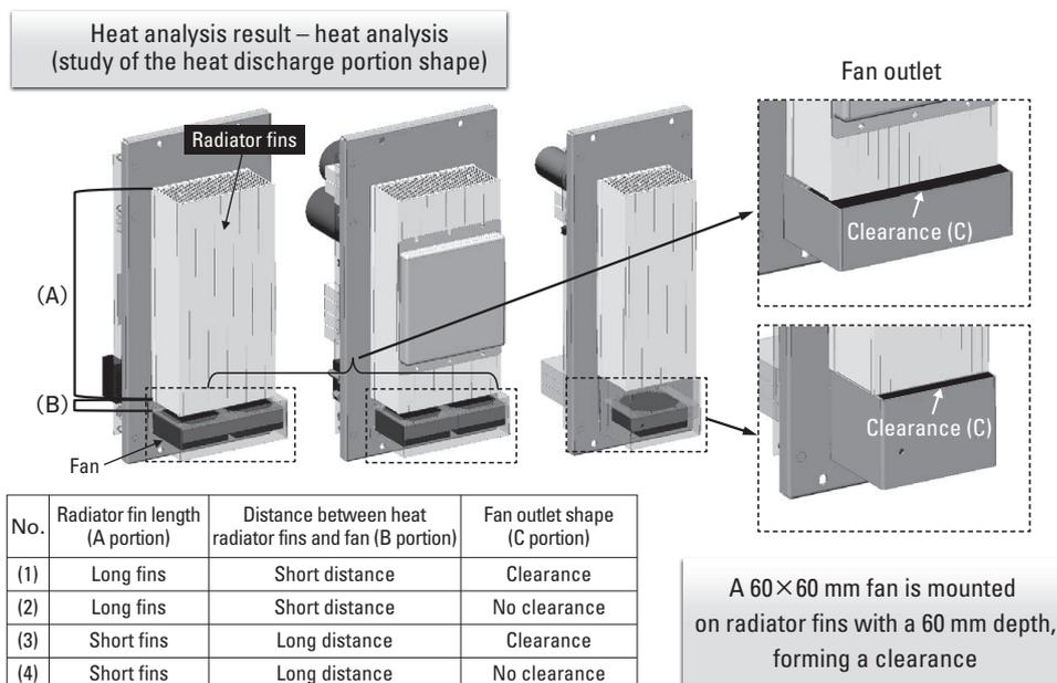
Fig. 6: Distance between radiator fins and cooling fan
