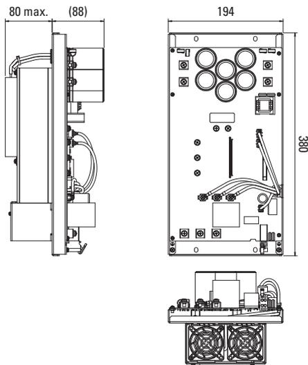
Fig. 4: Dimensions (Amplifier unit 150 A)
