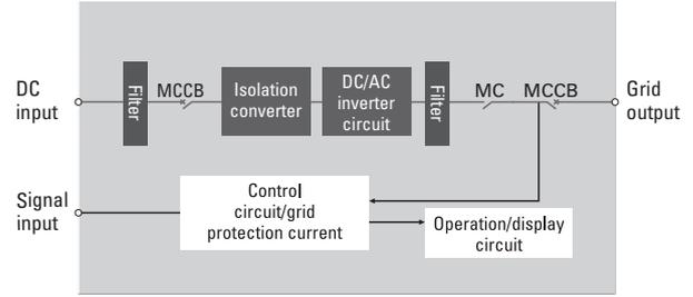
Fig. 3: Basic circuit configuration
