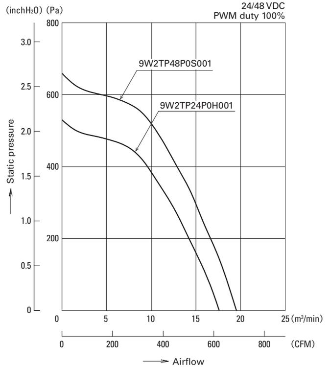
Fig. 6: Airflow vs. static pressure characteristics of the ø221 × 71 mm *San Ace 221W* 9W2T type
