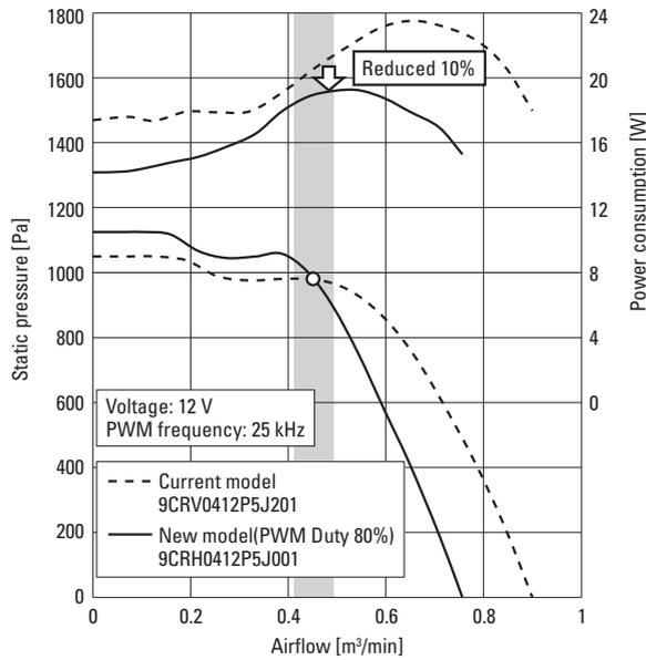
Fig. 9: Example of the airflow vs. static pressure characteristics (comparison with current model)
