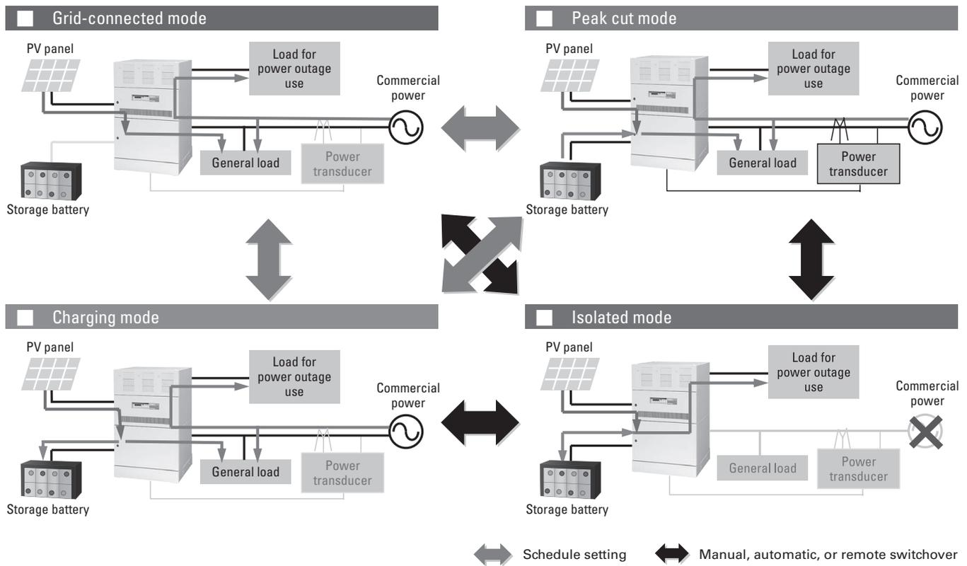
Fig. 2: Switchover between operation mode
