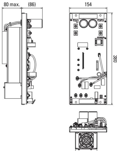
Fig. 3: Dimensions (Amplifier unit 75 A)
