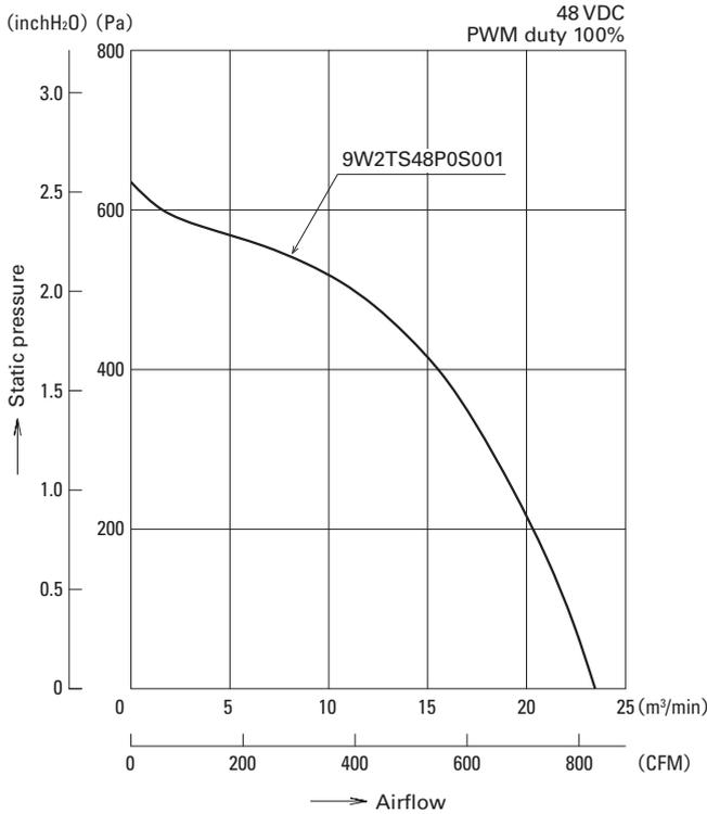
Fig. 5: Airflow vs. static pressure characteristics of the ø225 × 99 mm *San Ace 225W* 9W2T type
