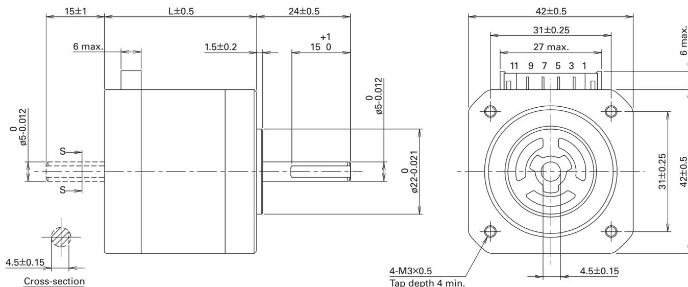
Fig. 2: External dimensions of the new model
