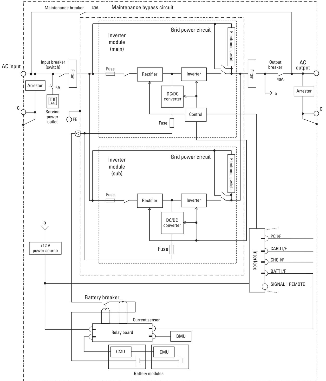
Fig. 3: Circuit diagram for the SANUPS N11B-Li (3 kVA)
