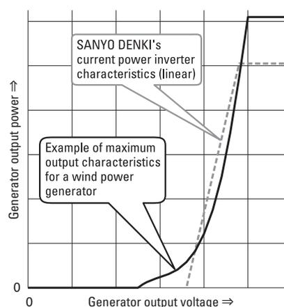
Fig. 1: Example of wind power generator output characteristics and the output characteristics of SANYO DENKI's current model
