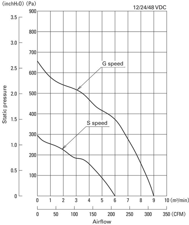
Fig. 5 Airflow vs. static pressure characteristics of the new models *San Ace 140L* and *San Ace 140W*
