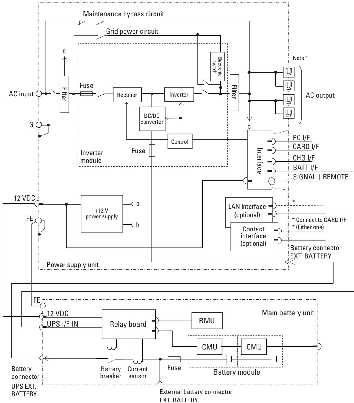
Fig. 3 Circuit diagram for the SANUPS N11C-Li (1.5 kVA)
