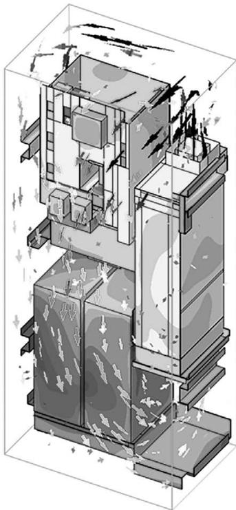
Fig. 6 Thermal fluid analysis model of the *SANUPS N11B-Li* (3 kVA)
