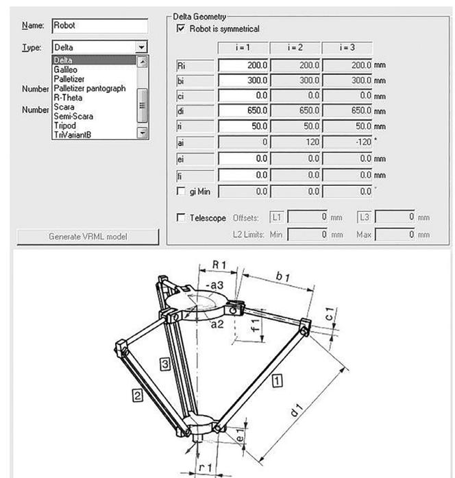
Fig. 1 Robot mechanism setting tool
