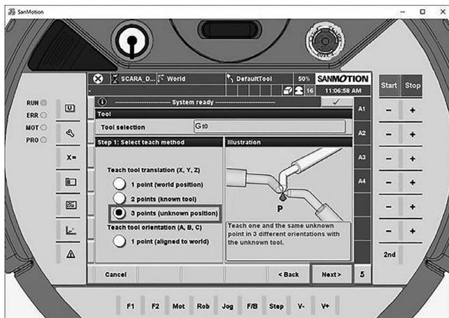
Fig. 3 Robot hand setting screen
