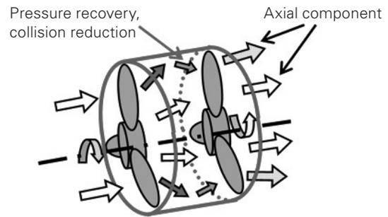
Fig. 7 Illustration of Counter Rotating Fan flow
