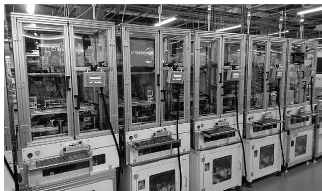
Fig. 5 Automatic inspection line for motors
