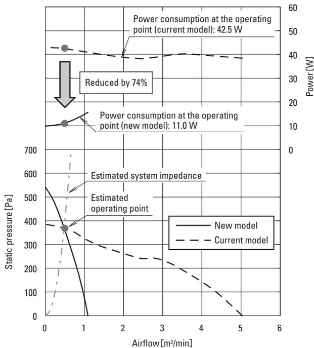
Fig. 9 Comparison of power consumption at operating point
