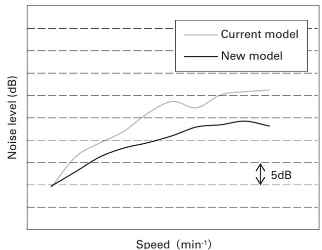
Fig. 7 Noise level comparison (54 × 54 mm 110 W motors, no-load)
