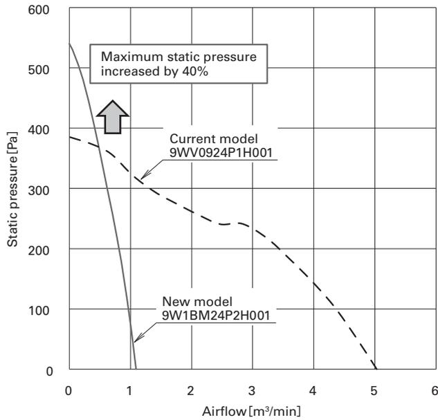
Fig. 8 Comparison of airflow vs. static pressure characteristics
