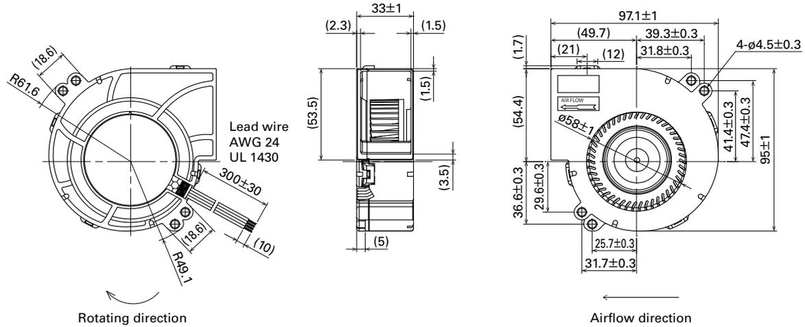
Fig. 2 Dimensions of the new model (unit: mm)
