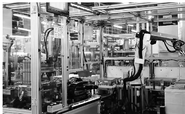
Fig. 2 Magnet bonding unit for 20 × 20 mm AC servo motors
