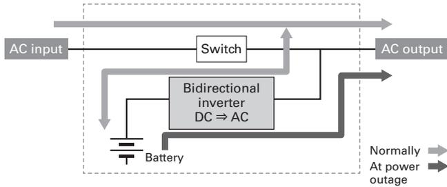
Fig. 5 Parallel processing topology
