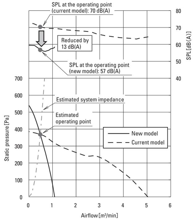
Fig. 10 Comparison of SPL at operating point
