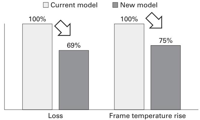
Note: Test conditions: Rated output (according to in-house heat dissipation conditions)
