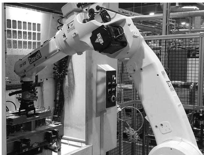
Fig. 4 Tandem operation of a robot and machine tool
