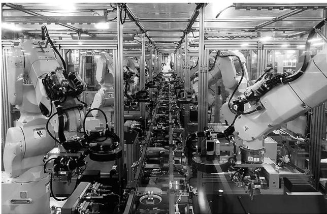
Fig. 6 Component insertion line with robots
