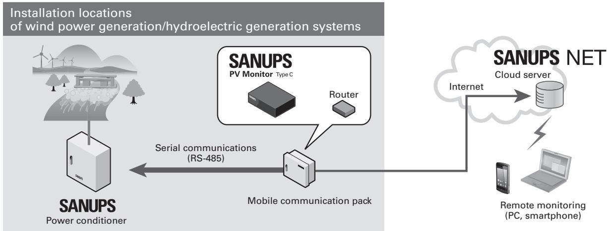
Fig. 5 Example of remote monitoring system configuration
