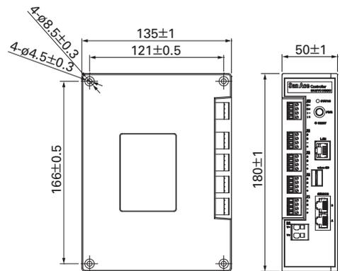
Fig. 3 *San Ace Controller* dimensions
