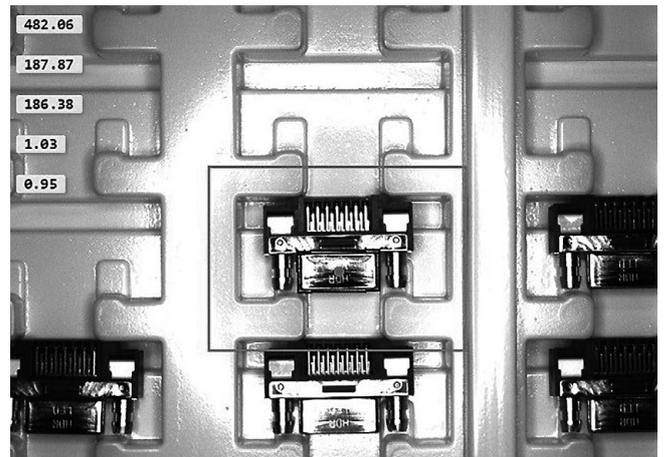
Fig. 7-1 Component coordinate detection using pattern matching
