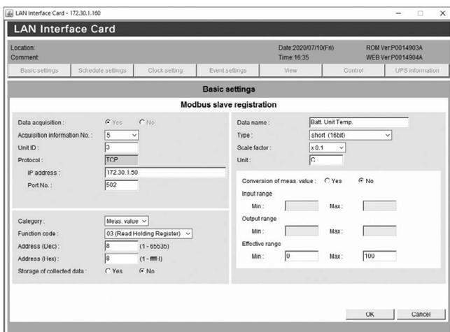
Fig. 6 Example screen for registering Modbus slave units
