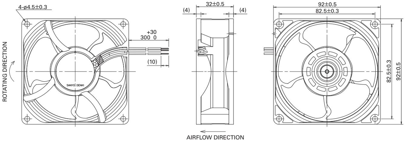
Fig. 9 Dimensions of *San Ace 92WF* (unit: mm)
