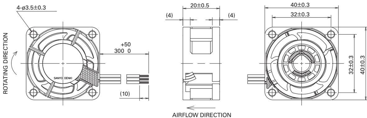
Fig. 6 Dimensions of *San Ace 40WF* (unit: mm)
