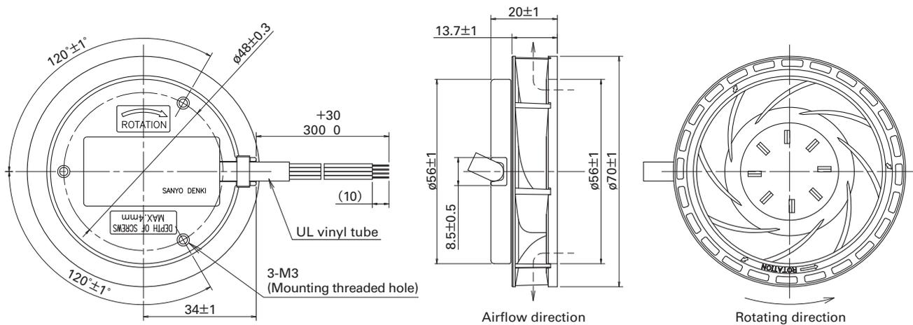
Fig. 2 Dimensions of the new model (unit: mm)
