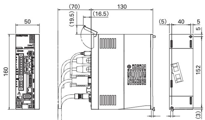
Fig. 4 Dimensions of the serial type 200 VAC, 30 A model
