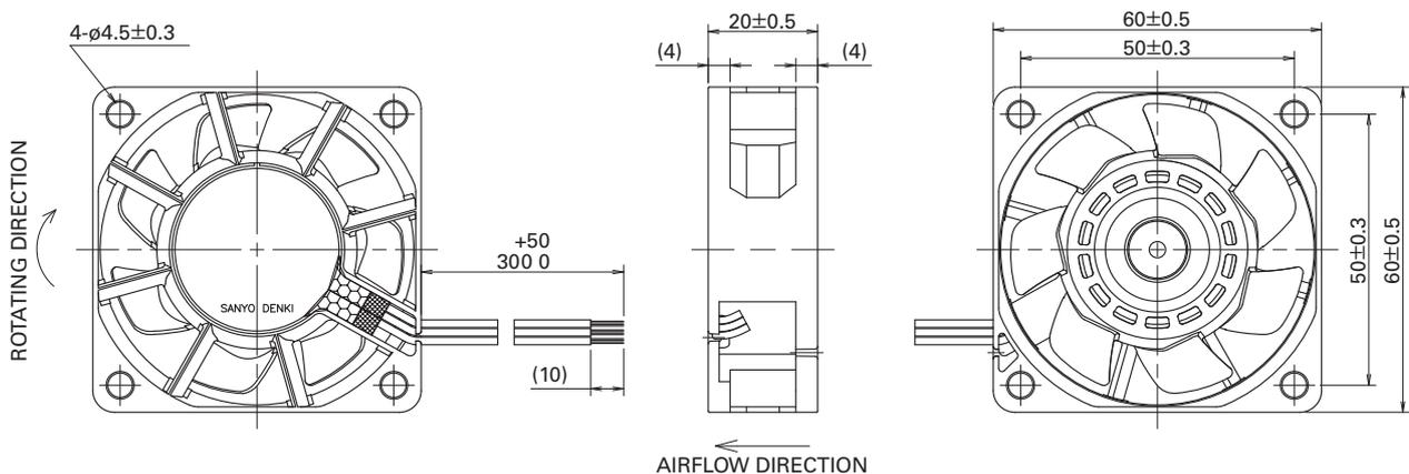
Fig. 7 Dimensions of *San Ace 60WF* (unit: mm)
