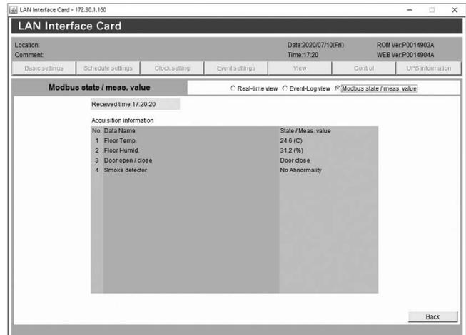
Fig. 7 Example screen for displaying Modbus slave unit information
