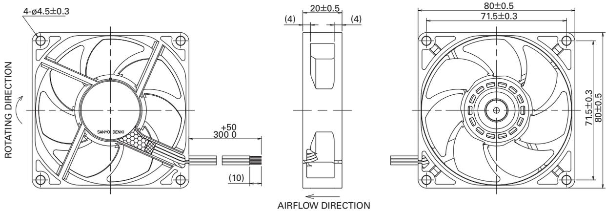
Fig. 8 Dimensions of *San Ace 80WF* (unit: mm)
