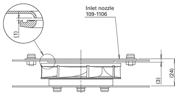
Fig. 4 Dimensions of new model with inlet nozzle installed (unit: mm)
