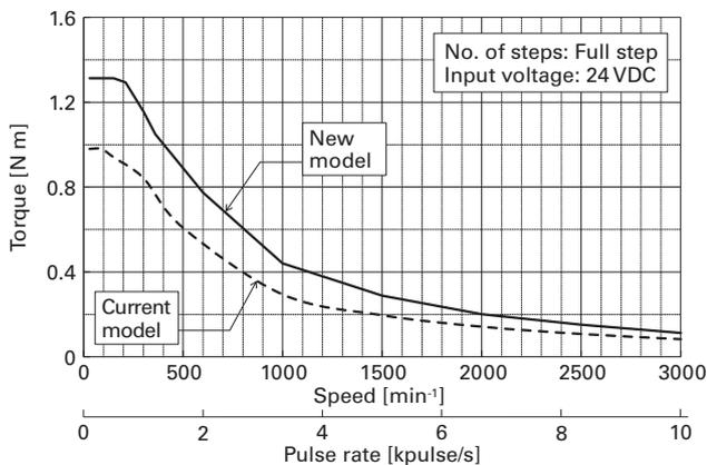
Fig. 3 Rotational speed vs. torque characteristics (SM2562C30B41)
