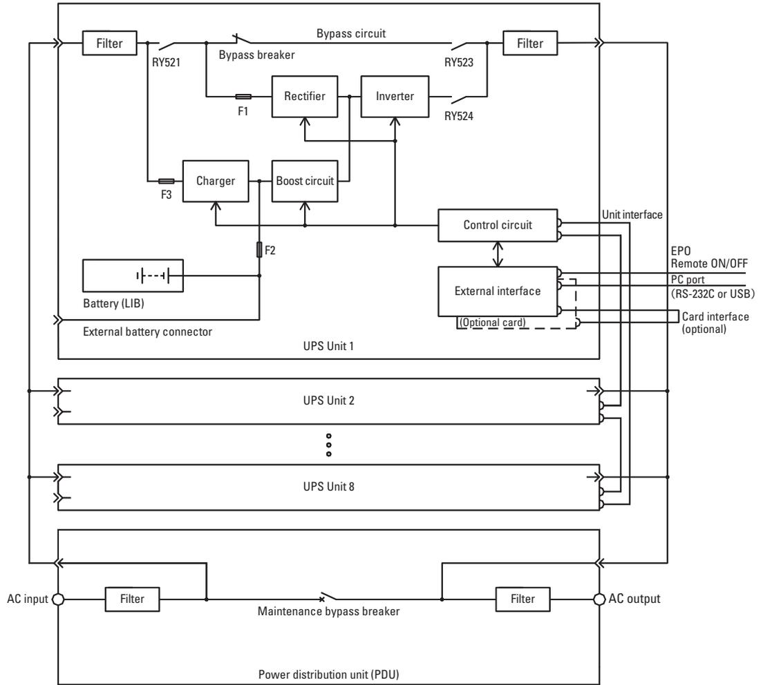
Fig. 6 A11M-Li system diagram
