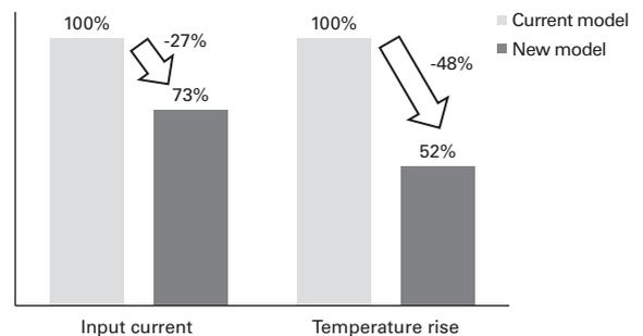
Fig. 4 Comparison of input current and temperature rise (SM2562C30B41)
