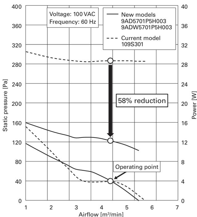
Fig. 10 Power consumption comparison between new and current models (100 V, 50 Hz)
