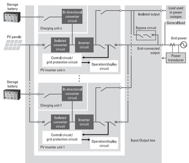
Fig. 4 Block diagram for grid-connected isolated charging type
