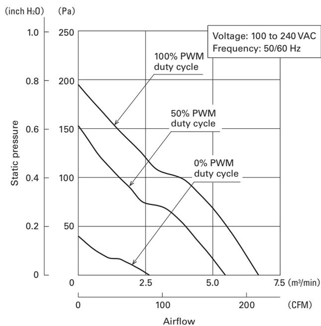
Fig. 5 Airflow vs. static pressure characteristics of new models
