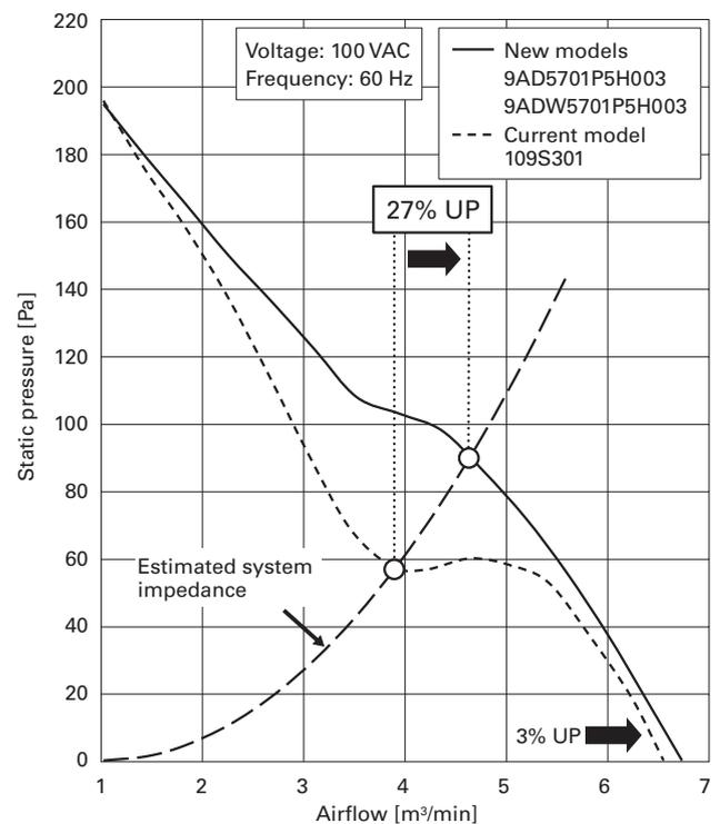
Fig. 8 Airflow vs. static pressure characteristics of the new and current models
