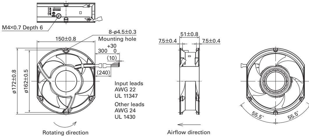
Fig. 4 Dimensions of the *San Ace 172AD 9ADW* type (Unit: mm)
