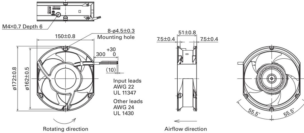
Fig. 3 Dimensions of the *San Ace 172AD 9AD* type (Unit: mm)
