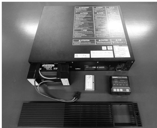
Fig. 8 Front panel and LIB
