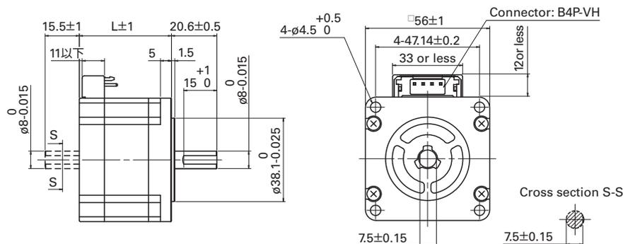
Fig. 2 Dimensions of the new model
