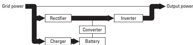
Fig. 3 The power supply path for the Double Conversion mode
