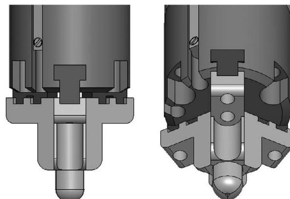
Fig. 9 Robot gripper finger
