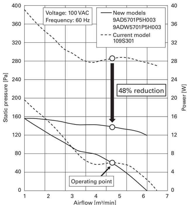
Fig. 9 Power consumption comparison between new and current models (100 V, 60 Hz)
