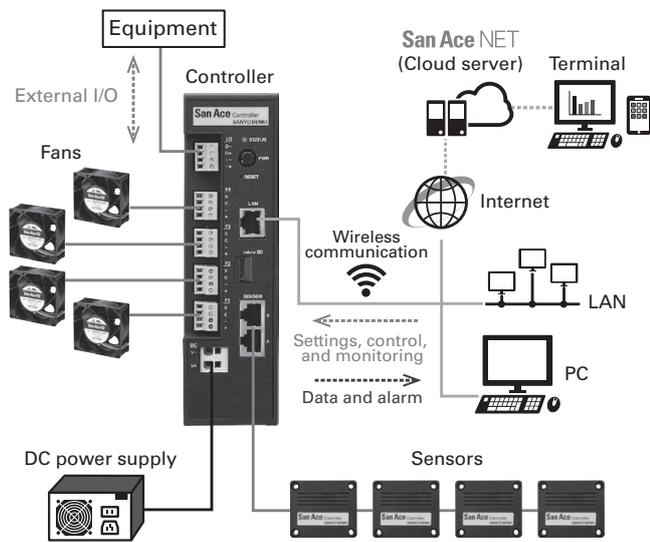
Fig. 4 *San Ace Controller* system configuration example
