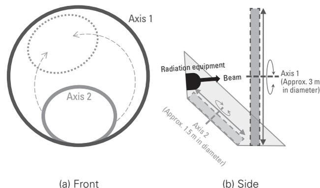
Fig. 5 Beam irradiation direction servo mechanism and size
