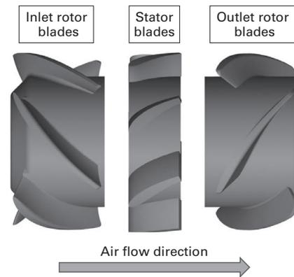
Fig. 2 Structure of our 40 × 40 × 56 mm Counter Rotating Fan
