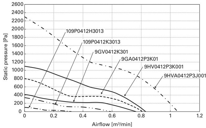
Fig. 1 Airflow vs. static pressure characteristics of our 40 × 40 × 28 fans
