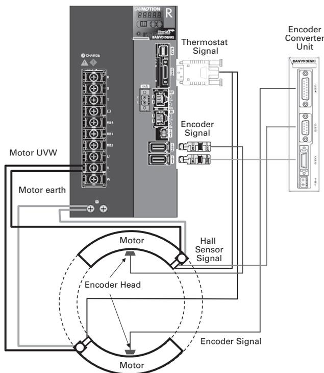
Fig. 6 Image of encoder signal redundancy
