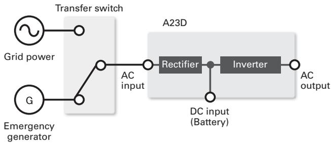
Fig. 5 Emergency power supply system
