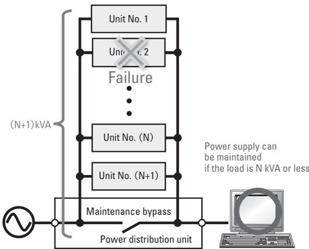
Fig. 8 Parallel redundant system with *SANUPS A11N, A11M(-Li)*
