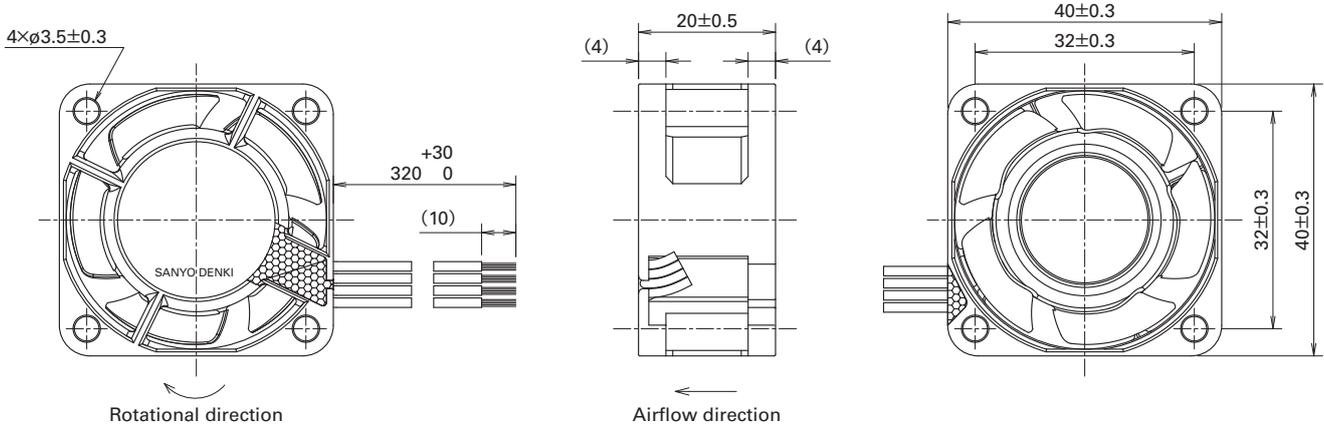
Fig. 4 Dimensions of 40 × 40 × 20 mm *San Ace 40W 9WPA* type (Unit: mm)
