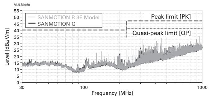
Fig. 7 Radiated emissions (10 m, horizontal)
