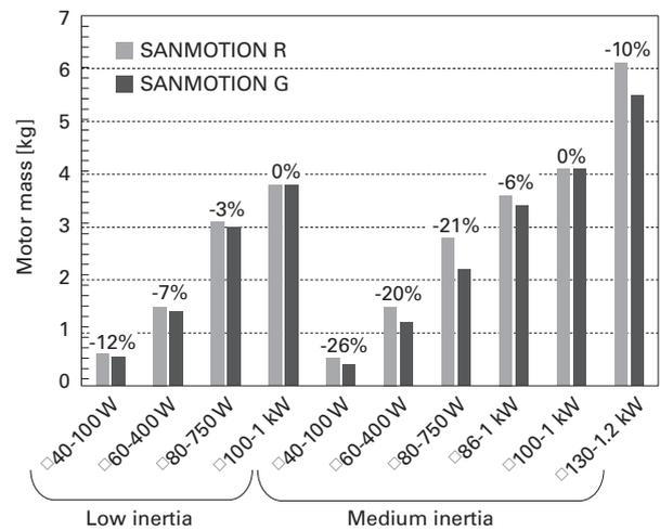
Fig. 9 Comparison of motor mass (Without holding brake)
