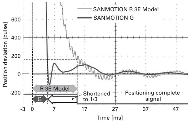
Fig. 6 Positioning characteristics
