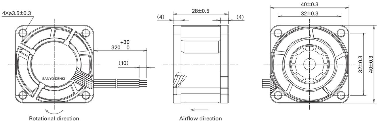
Fig. 5 Dimensions of 40 × 40 × 28 mm *San Ace 40W 9WPA* type (Unit: mm)
