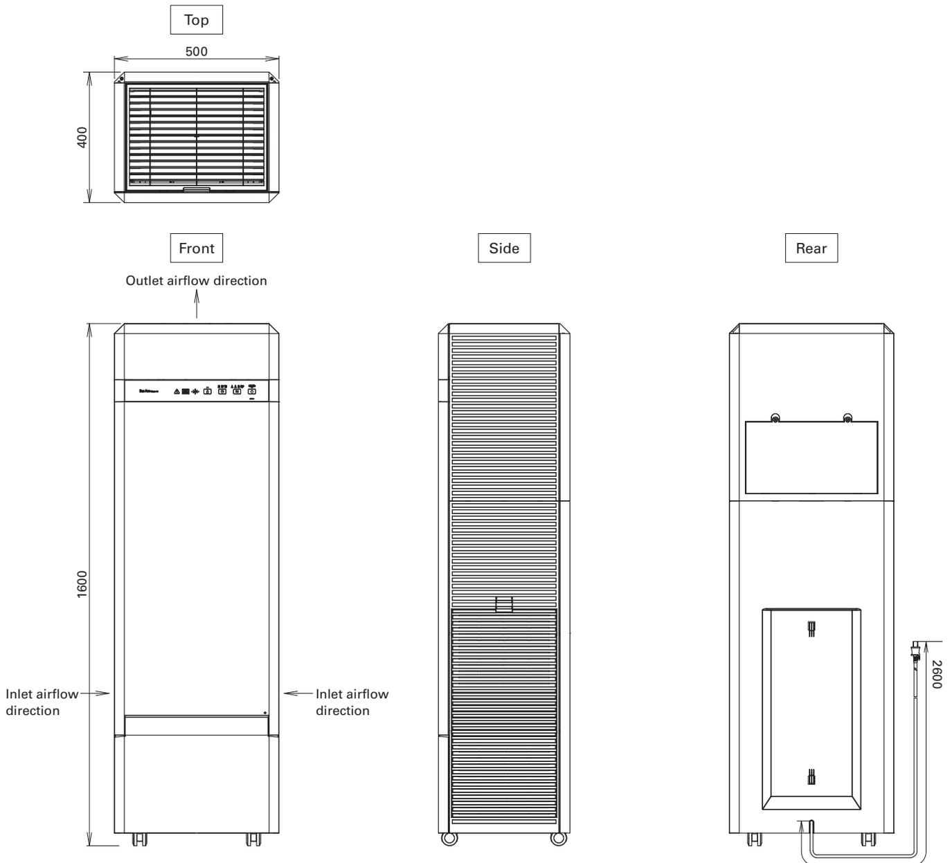
Fig. 4 Dimensions of *San Ace Clean Air* 9AP type (Unit: mm)
