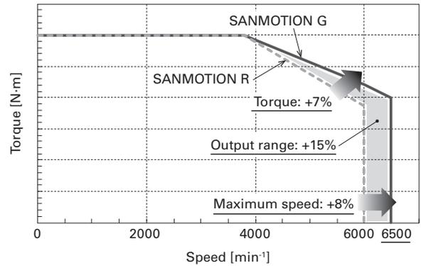
Fig. 4 Comparison of servo motor torque-speed characteristics
