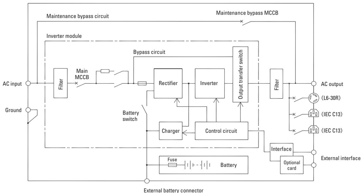
Fig. 8 Circuit block diagram (single unit type, 5 kVA)
