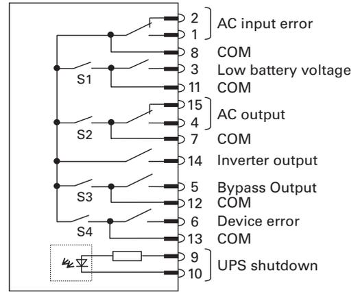
S1~S4 : Dry contact signal isolation switches
