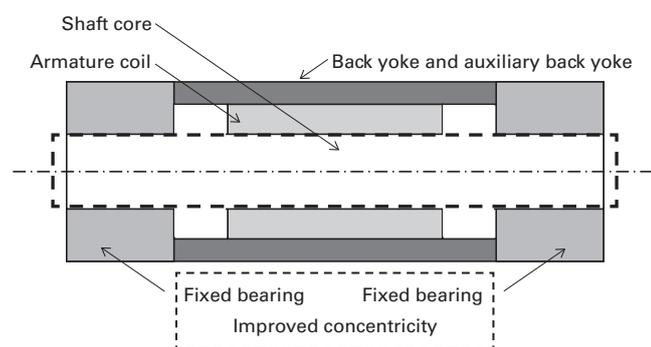
Fig. 6 Cross section view of new product's stator
