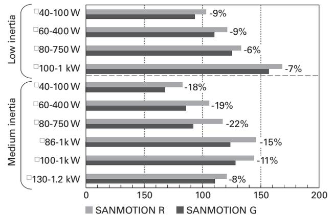
Fig. 8 Comparison of motor length (Without holding brake)
