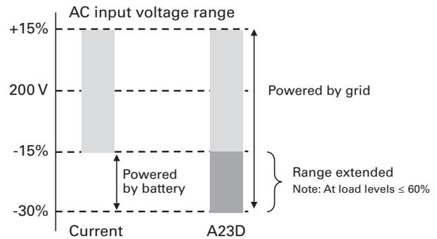
Fig. 4 Wide input voltage range
