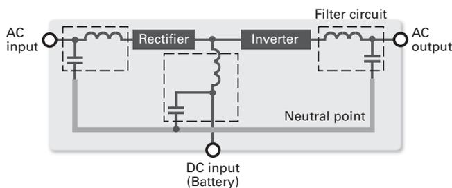
Fig. 3 Simplified A23D circuit block diagram
