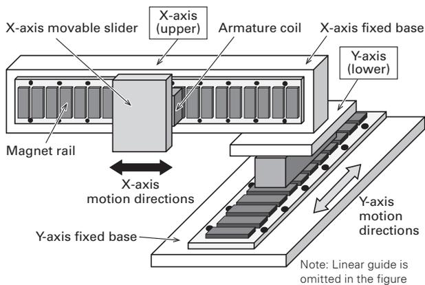
Fig. 11 Illustration of XY cartesian robot mechanism
