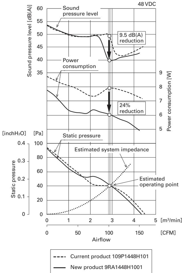
Fig. 6 Noise level and power consumption comparison
