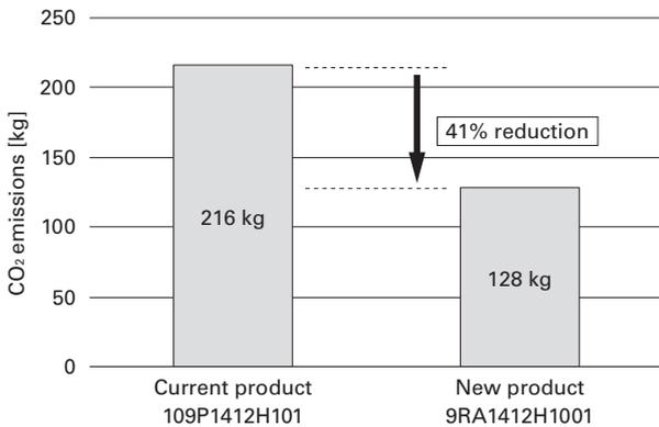
Fig. 7 CO<sub>2</sub> emissions comparison based on our life cycle assessment calculation software (40,000-hour continuous operation in free air)
