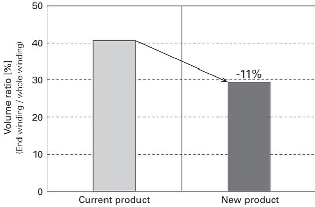
Fig. 6 Comparison of winding volume
