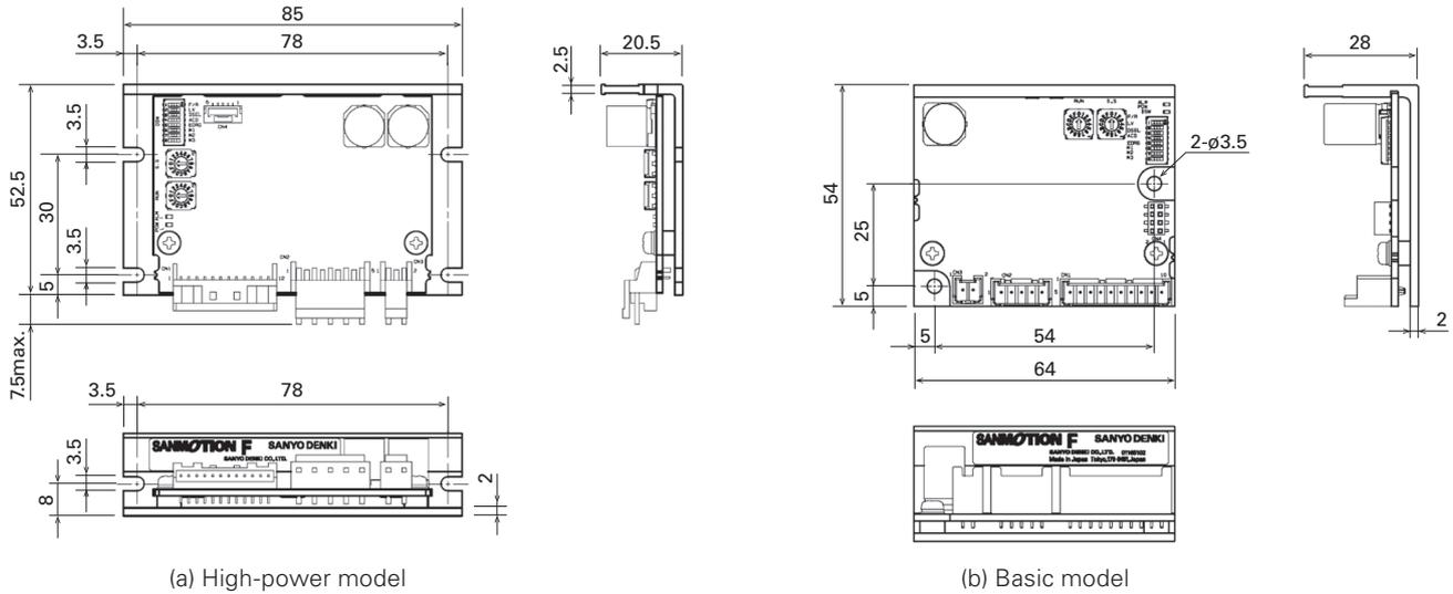
Fig. 2 Dimensions of new models (unit: mm)
