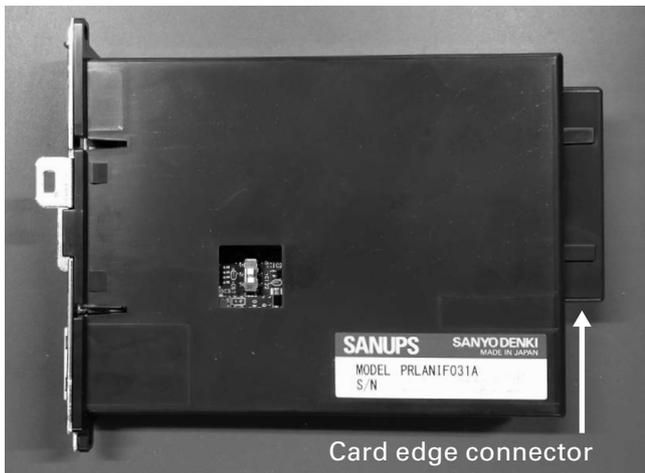
Fig. 5 Card edge connector of the LAN Interface Card
