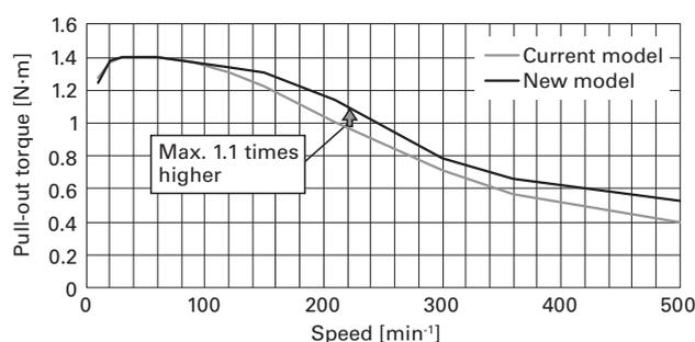
Fig. 4 Pull-out torque characteristics of basic model
