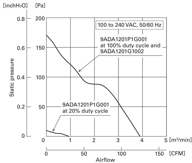
Fig. 5 Airflow vs. static pressure characteristics of 9ADA1201P1G001
