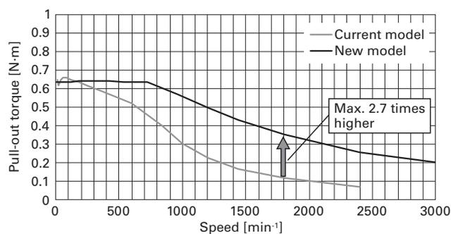
Fig. 3 Pull-out torque characteristics of high-power model
