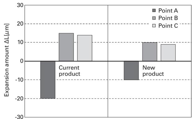
Fig. 12 Thermal expansion in moving slider (analyzed results)
