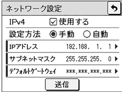
Fig. 4 Screen example of IP address settings for the SANUPS A23D
