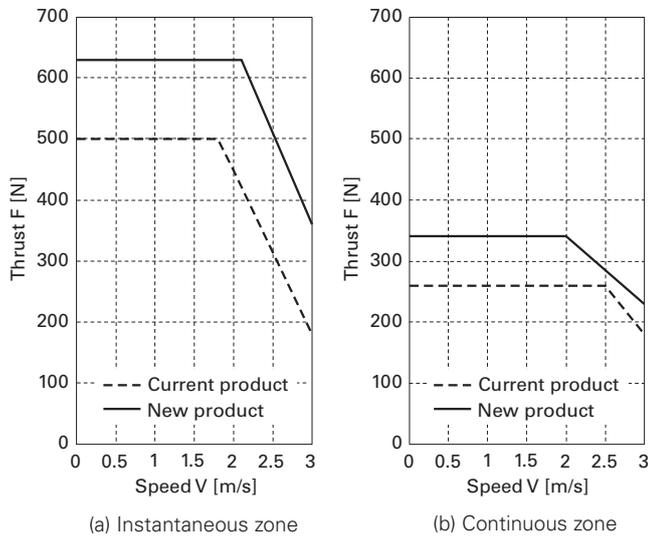
Fig. 10 Thrust vs speed characteristics (at 200 V input)
