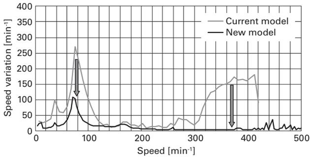
Fig. 5 Comparison of motor speed variation characteristics
