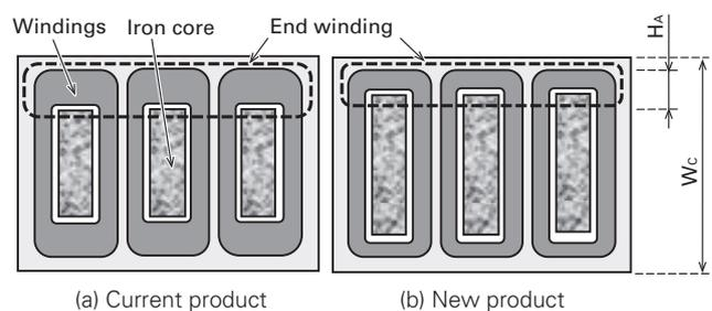
Fig. 5 Comparison of winding structure (reduced end winding)
