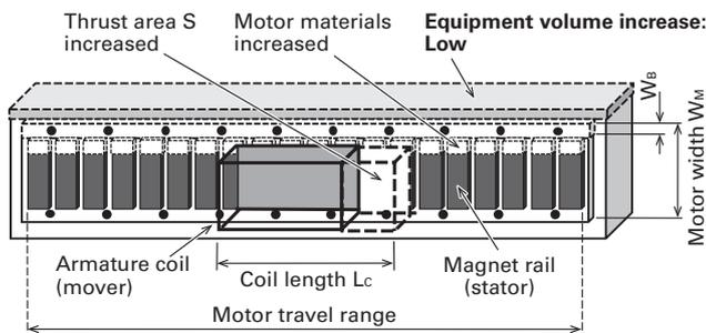
Fig. 3 Installation example of new linear servo motor
