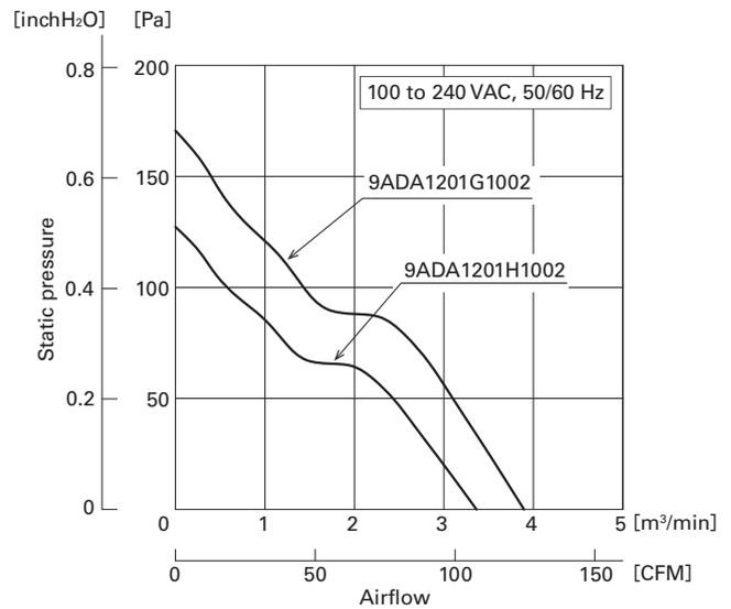
Fig. 6 Characteristics comparison between 9ADA1201G1002 and 9ADA1201H1002
