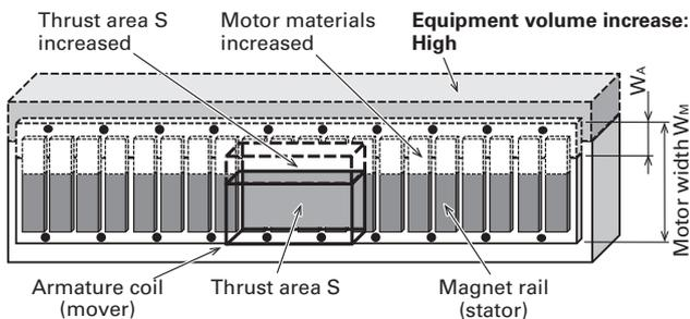
Fig. 2 Installation example of current linear servo motor
