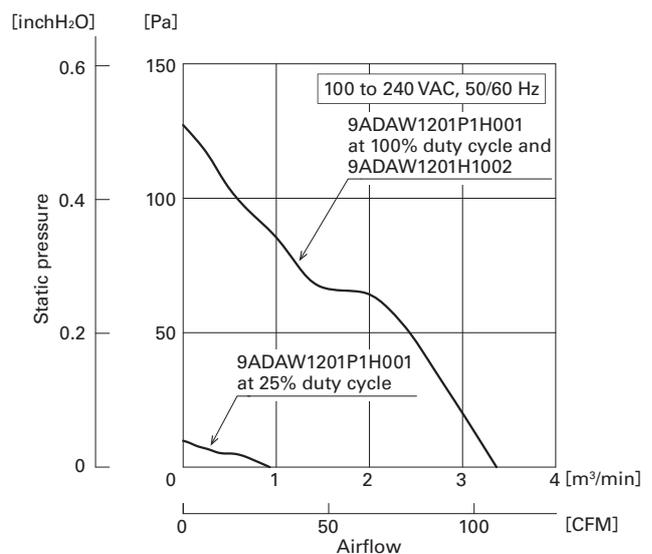
Fig. 7 Airflow vs. static pressure characteristics of 9ADAW1201P1H001
