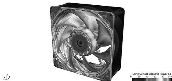
Fig. 6 Simulation-based sound source analysis example
