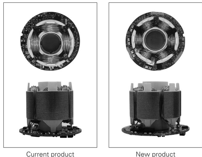
Fig. 4 Motors of the new and current products
