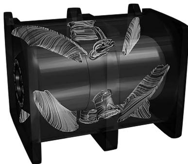
Fig. 6 Simulation example (Airflow of the new product)
