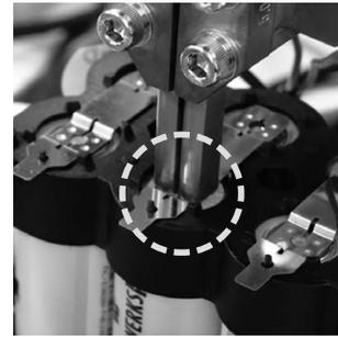
Fig. 8 Resistance welding
